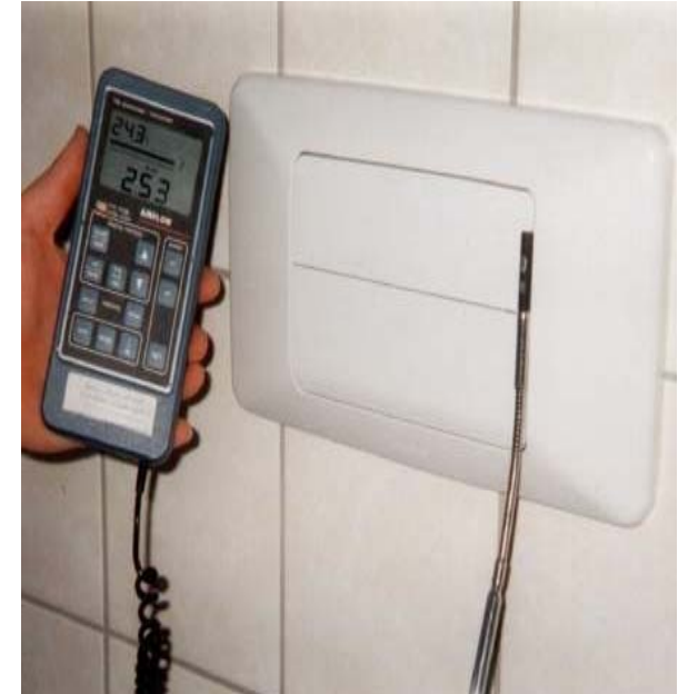
BlowerDoor final measurement according to ISO 9972 or DIN EN 13829
