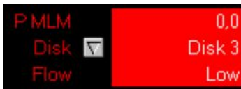
Fig. 4.35: Low – Disk pressure differential is too low
