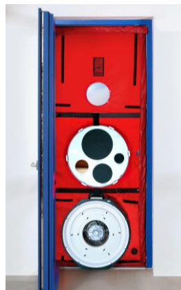
Fig. 3.2: Installed field check ring and BlowerDoor Standard fan
