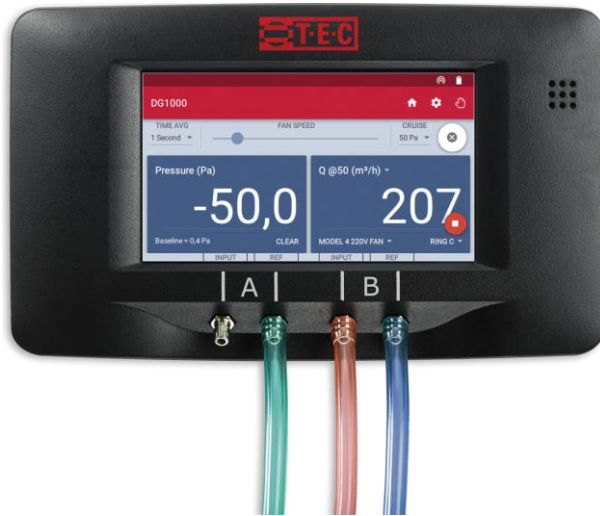
Fig. 4.28: Tube connection at DG-1000
