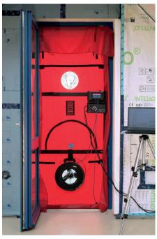
With the pressure gauge DG-1000 and the software TECTITE Express, the BlowerDoor measurement is carried out with highest accuracy automatically, semi-automatically or manually on the laptop according to ISO 9972 and EN 13829. When performing quality assurance tests, the BlowerDoor fan is controlled directly from the DG-1000 and a 1-point test is conducted to detect leakages.
