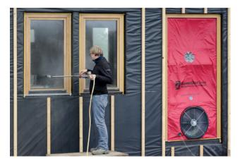
Ideally, the measurement should be conducted in combination with a Minneapolis BlowerDoor measuring system like BlowerDoor Standard or BlowerDoor Mini-Fan. Negative pressure tests are particularly suited to detect even small leakages. The tests can be further supported by using a thermal-imaging camera. For easy transport, the portable SPRAY BAR system
